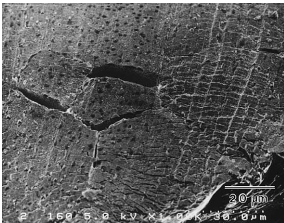
Fig. 8. Scanning electron micrograph of the outer surface of a specimen implanted with 600 appm helium at 600 °C and tensile-tested at 600 °C. The stress direction was close to vertical with respect to the figure.
